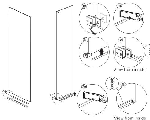
Vertical profile can be adjusted 10mm, When the glass is fully inserted into the vertical profile, bottom U channel need to be cut 10mm, when the glass isn't fully inserted into the vertical profile, bottom U channel need to be cut accordingly
