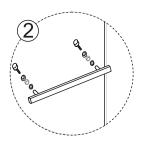
Ensure wall profiles are plumb. Adjust enclosure to be square and level. Wall post and profile should be adjust to square the doors and Ensure open door smooth.
