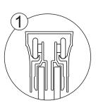
Ensure wall profiles are plumb. Adjust enclosure to be square and level. Wall post and profile should be adjust to square the doors and Ensure open door smooth.
